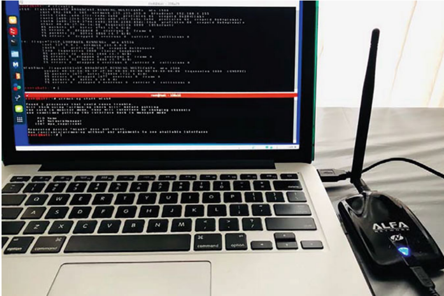
Fig. 7 Wireless adapter WLAN0 set to monitor mode to sniff data packets
