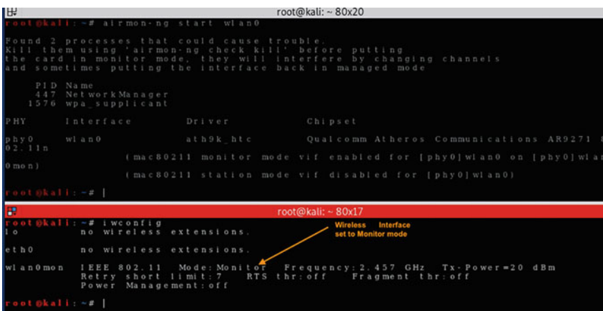
Fig. 8 Wireless interface in monitor mode
