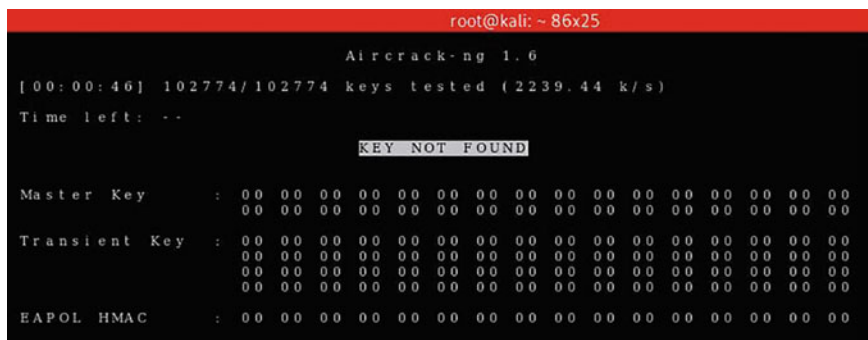
Fig. 17 Password not found in brute force cracking of station/smartphone password
