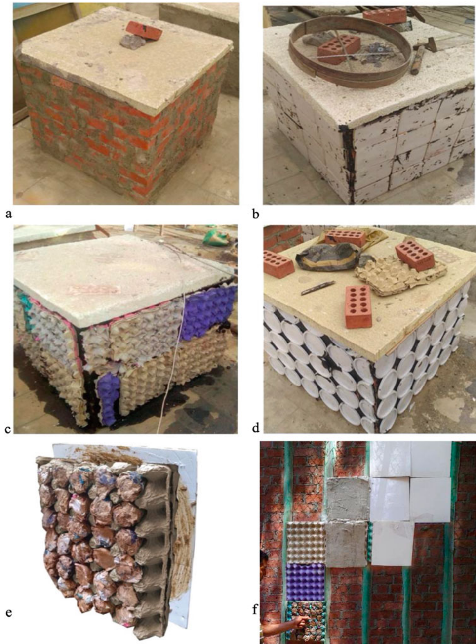
Fig. 7 The images represent the control experiment chamber (no insulation) and the 4 types of waste insulation developed for monitoring. a Control experiment chamber; b Styrofoam insulation; c Egg tray cardboard insulation; d Polypropylene insulation, and lastly. e a composite of compressed egg trays filled with cardboard mache and a bottom Styrofoam layer. f One further trial and error process that experimented with reusing waste plastic corrugated sheets as mullions for the panels to substitute the expensive Adibond 65 adhesive
