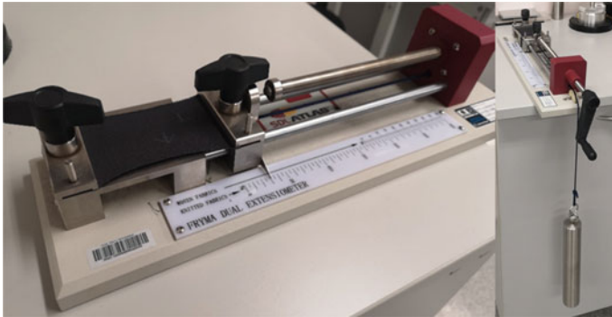
Fig. 21 SDL Atlas Fryma fabric extensometer
