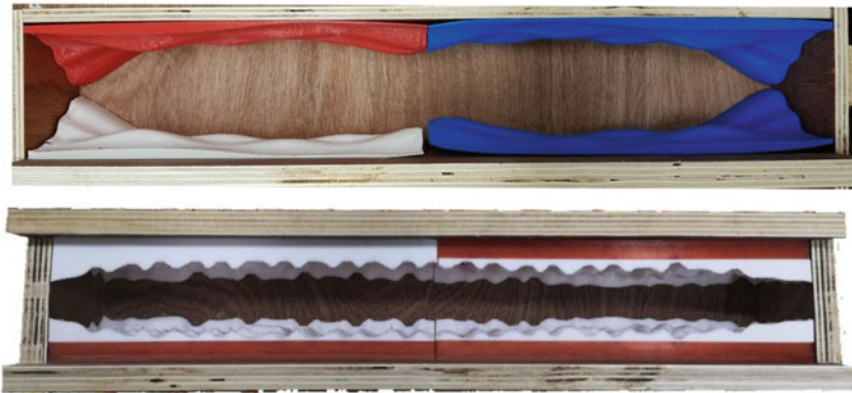
Fig. 9 Formworks structures consisting of PLA 3D printed parts. Formwork of DS 2 (top) and formwork of DS 3 (bottom)
