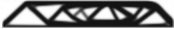
Fig. 1 Material optimization based on TO extracted from the TopOpt plug-in for the case study 6
