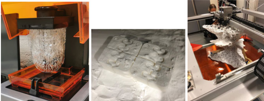
Fig. 7 From left SLA (Stereo Lithography), SLS (Selective Laser Sintering), and FDM (Fused Deposition Modelling) (Photo Steinar Killi)
