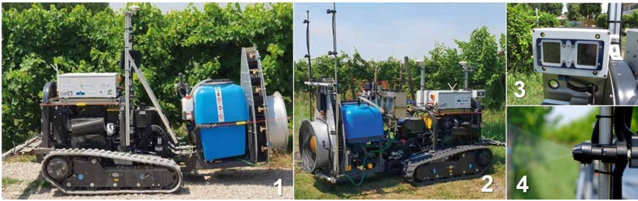
Fig. 1. The first prototype (1), operating at “Azienda Giorgio Pantano”, in the configuration of the first year of activity; the second prototype, operating at “Terre Grosse” (2) with the stereo cameras for canopy inspection (3) and the Pulse Width Modulation (PWM) nozzles (4).
