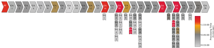
Fig. 8 Visualization of service time (red color scale) on the general assembly line and subassembly stations. The major bottleneck in the process is formed by the general assembly station GA16
