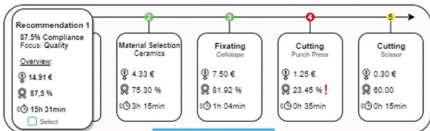
Fig. 9 Illustration of a recommended process configuration from the FRP process chain planning tool with a global evaluation of the whole chain on the left and local information on possible problems on the right
