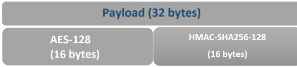
Fig. 6. Payload from devices to server S containing encrypted data and authentication code
