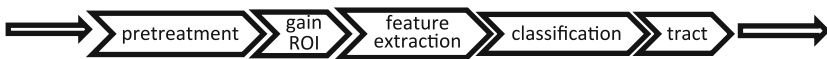
Fig. 1. The general sequence of the main modules in the traditional pedestrian detection
