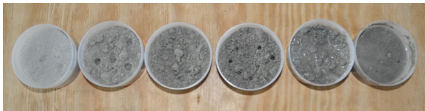
Fig. 15.18 Six frozen samples of NU-LHT-2M with increasing volumes of water added. Each container has a diameter of 7.2 cm and a height of 3.3 cm. Source Pitcher et al. (2016)
