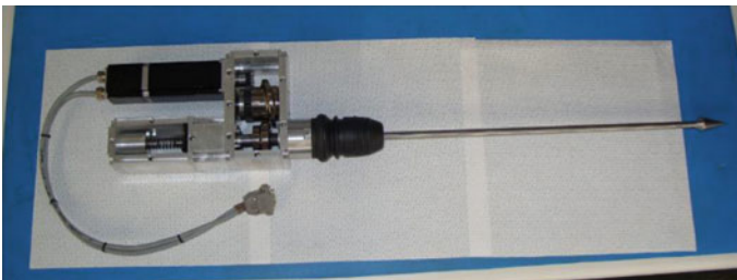
Fig. 15.15 The Honeybee Robotics percussive cone penetrometer. Source Mantovani et al. (2016)
