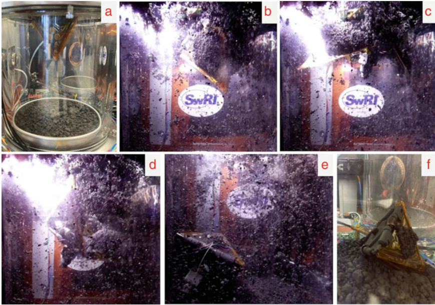
Fig. 24.9 The Clockwork Starfish asteroid surface sampling technology demonstration before (a), during (b–e) and after (f) a microgravity flight aboard Blue Origin’s New Shepard (NS-13) suborbital flight (Images courtesy project PI, Dr Daniel Durda)
