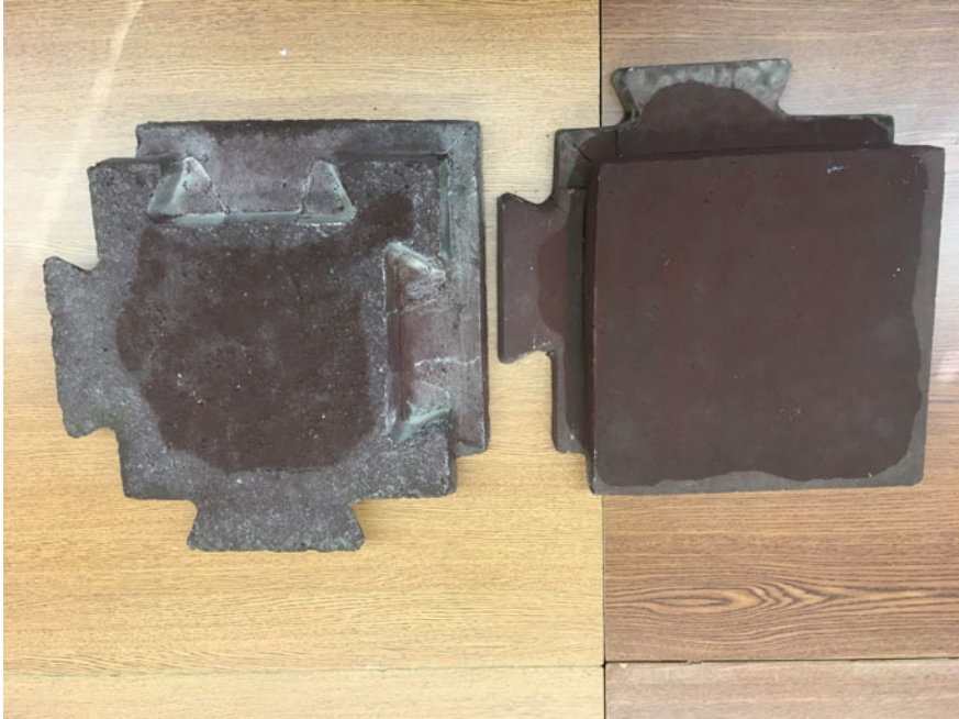
Fig. 13.2 Interlocking pavers made with Hawaiian sintered basalt
