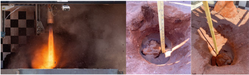
Fig. 14.9 Pulse 2 is lower thrust, simulated here by increased engine height and far field plume effects (left) to break up the icy blocks and excavate more regolith. This leaves an enlarged crater (center and right) that grew 393% over the volume of the crater in Pulse 1. This demonstrates the effectiveness of chained pulses to break up and transport frozen regolith
