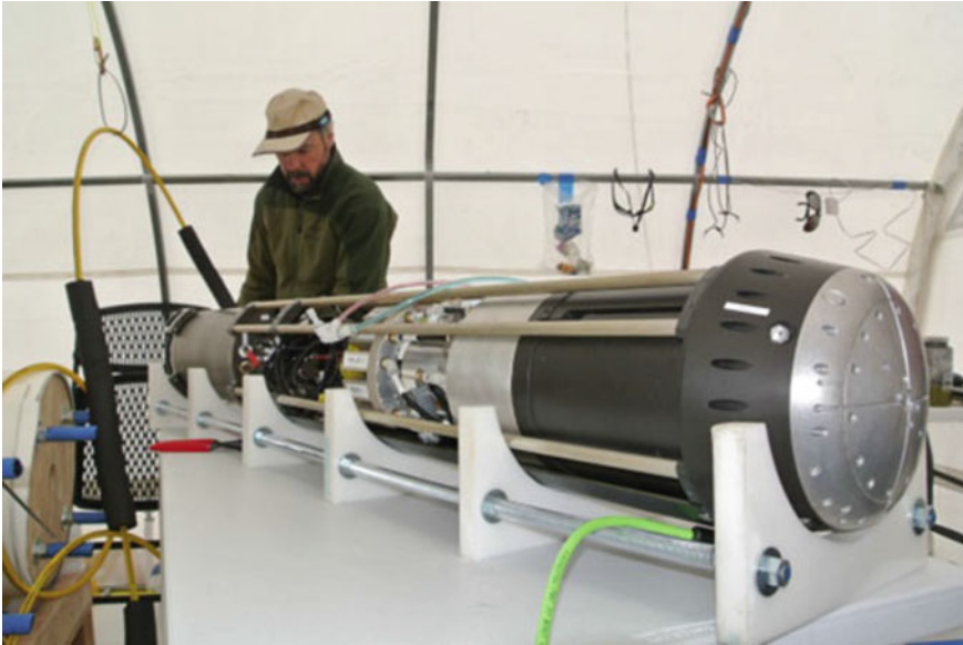
Fig. 29.10 The VALKYRIE probe during a field test on Matanuska glacier in Alaska, 2014, from Stone et al. (2018, p. 81)
