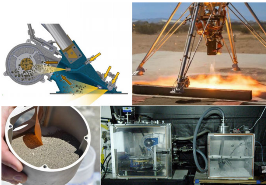
Fig. 14.13 The PlanetVac pneumatic system schematic (upper left) and test conditions (upper right). The regolith simulant sample gathering results from tests with Masten’s rocket (lower left), and the laboratory testing equipment at Honeybee Robotics (lower right)
