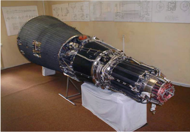
Fig. 29.5 Nuclear power plant for space applications “TOPAZ” (from Kraus and Shabalin 2013)
