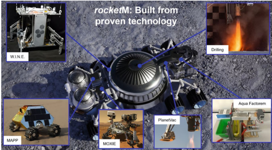
Fig. 14.4 Main hardware components of the rocketM rover-mounted system
