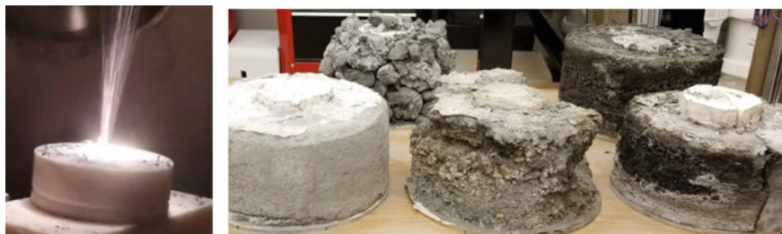
Fig. 10.4 Left: asteroid simulant spalling under a concentrated sunlight simulator. Right: Various densities, water concentrations, and structures of asteroid simulant. Source Colorado School of Mines
