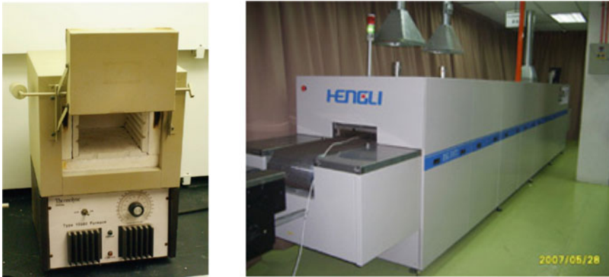
Fig 12.5 (left) A typical furnace used for sintering ceramics (Source David Harvey, CC BY-SA 4.0 https://creativecommons.org/licenses/by-sa/4.0 , via Wikimedia Commons); (right) A conveyor furnace for continuous sintering of many parts
