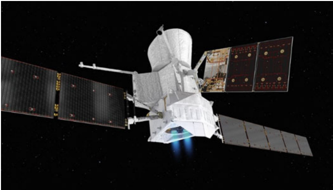
Fig. 8.2 BepiColombo spacecraft in cruise configuration. The Mercury Transfer Module with its two large solar wings carries the Mercury Planetary Orbiter (middle with one solar wing) and the Mercury Magnetospheric Orbiter, nicknamed Mio, hidden inside the solar shield
