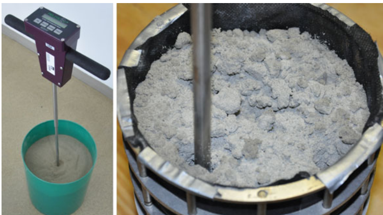
Fig. 15.19 The manual field penetrometer and measurement technique in a frozen NU-LHT-2M sample. Source Pitcher et al. (2016)
