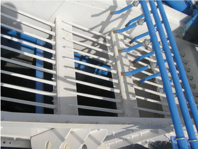
Fig. 11.11 Example of a grizzly screen used to filter out larger rock sizes. Photo by Peter Craven, Creative Commons CC-BY-2.0
