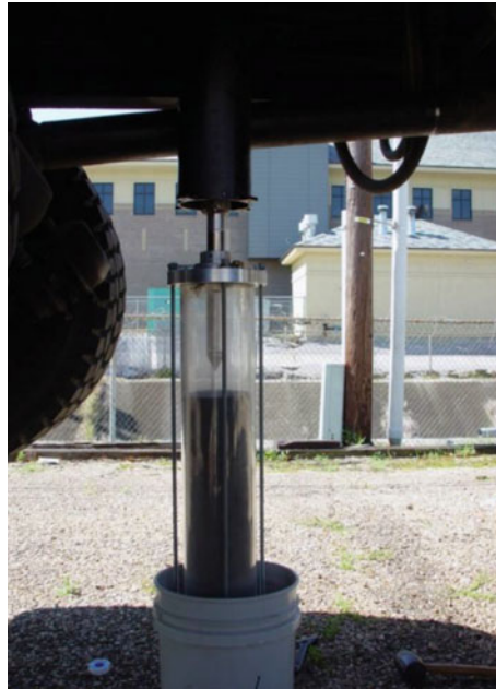
Fig. 15.28 The testing set-up for CPT measurements in JSC-1A, showing the large-diameter truck-mounted penetrometer and the relatively narrow cylindrical testing container. Source Cil (2011)
