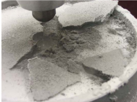
Fig. 15.24 Close view of a sample immediately after indentation, showing some of the chips and the fines produced. Source Gertsch et al. (2008)
