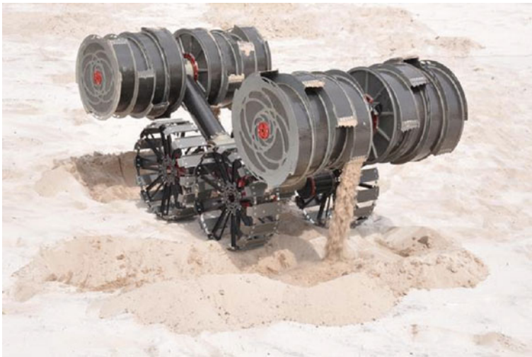
Fig. 11.10 NASA Regolith Advanced Surface Systems Operations Robot (RASSOR) Excavator 2.0 Prototype during testing. Credit NASA Kennedy Space Center, Swamp Works
