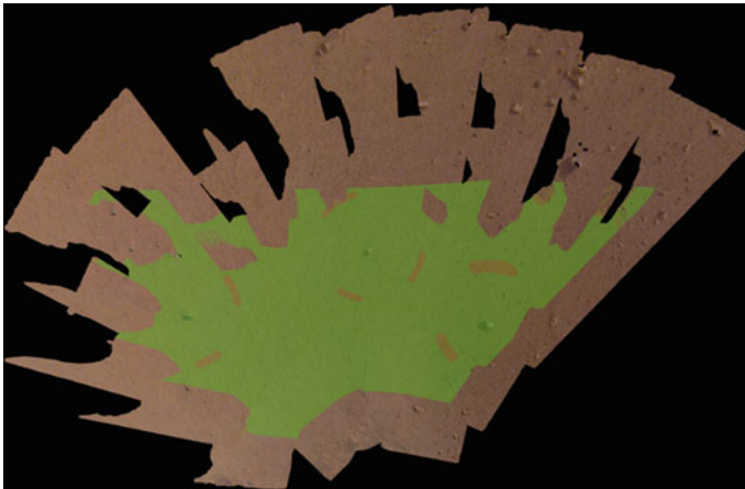
Fig. 21.13 Sol 12 orthorectified projection of the InSight Deployment Workspace with WTS “instrument roughness” overlaid. Green pixels represent locations that pass all of the instrument placement criteria, orange indicates one requirement has been violated, and red means at least two criteria are violated
