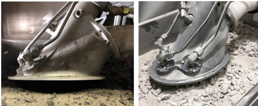
Fig. 10.1 Bracketing use cases for the PlanetVac system. Left: tests in dense, rocky simulant. Right: tests in low-density aircrete. Source Courtesy of Honeybee Robotics
