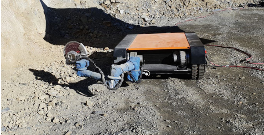
Fig. 31.8 OffWorld's Diggerbot in the field (used with permission of OffWorld)
