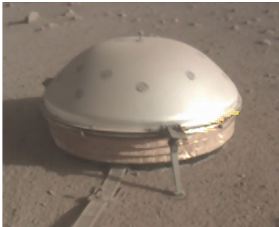
Fig. 21.24 The wind and thermal shield (WTS) on the Martian surface on Sol 394. The SEIS is underneath the WTS, and the SEIS tether can be seen protruding from underneath the WTS skirt
