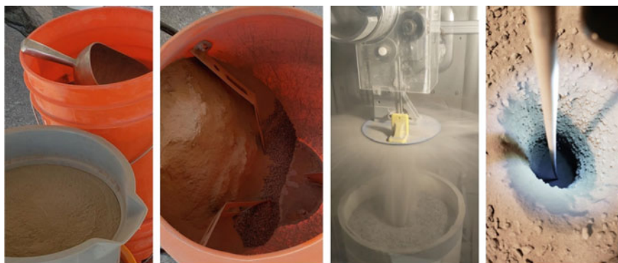
Fig. 10.2 Left to right: simulant materials in buckets before combination, mixing simulant base materials for desired geotechnical properties, testing in a thermal vacuum environment using custom simulant, bore hole after test. Source Honeybee Robotics
