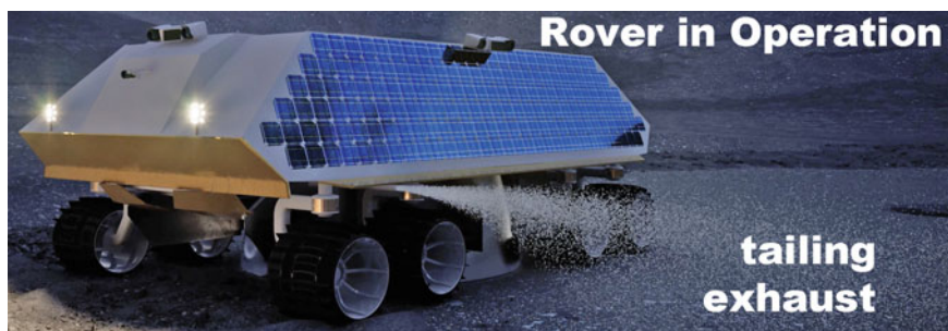
Fig. 14.16 Rover in operation exhibiting tailings exhaust
