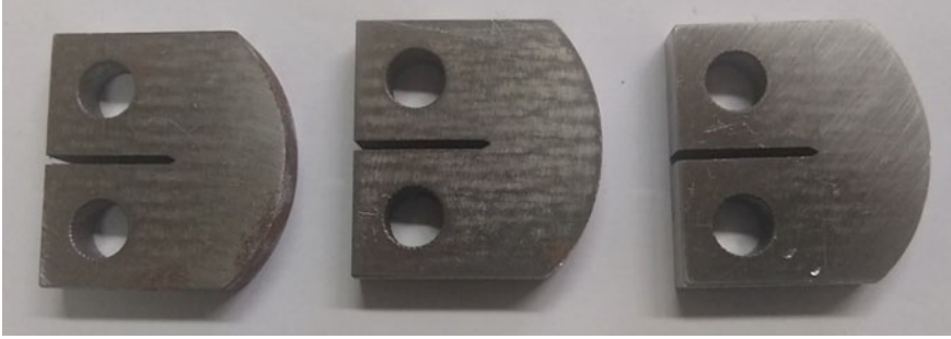
Fig. 1.1 C(T) specimens for different regions of the welded joint
