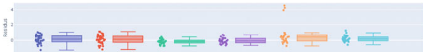
Fig. 21.5 Box plot of residuals for steel for: (i) Basquin (log-normal distribution), (ii) Basquin (2-parameter Weibull), (iii) Castillo and Fernández-Canteli, (iv) Stüssi, (v) Strohmeier (fatigue limit) and (vi) Strohmeier (number of cycles)
