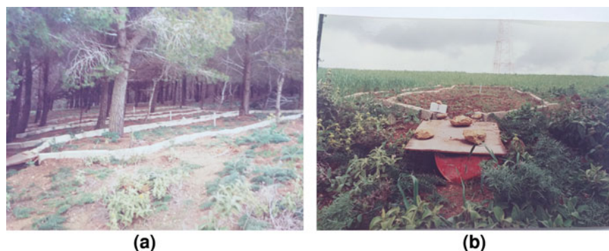
Fig. 2 Soil erosion plots for soil loss measurements at the study locations; (a) Alhamama, and (b) Shahat
