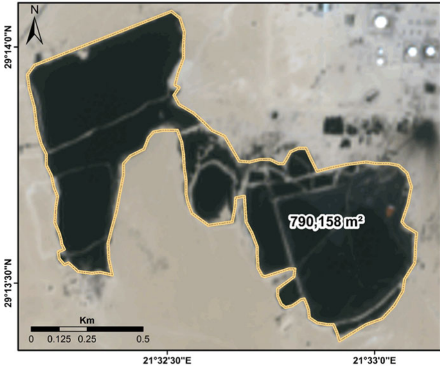
Fig. 10 Landsat 8 acquired in 2018 shows Nafoora Oil Field CPS 1 and 2 pit which shows the change in the pit size and volume which come to be about 790,158 m 2
