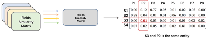
Fig. 2. The method of finding the corresponding entities in the standard table and physical table based on the fused similarity matrix
