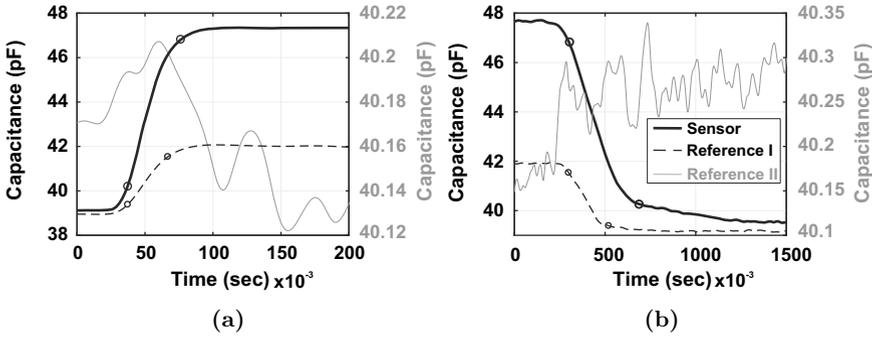
**Fig. 3.9** Comparison between the measured dynamic response of RH capacitive sensor, reference I and reference II of Fig. 3.6. **a** Adsorption and rise time, **b** spontaneous desorption and fall time of RH sensor, reference I and reference II. The value of reference II capacitance is near-stable and plotted on the scaled y-axis on the right-hand side
