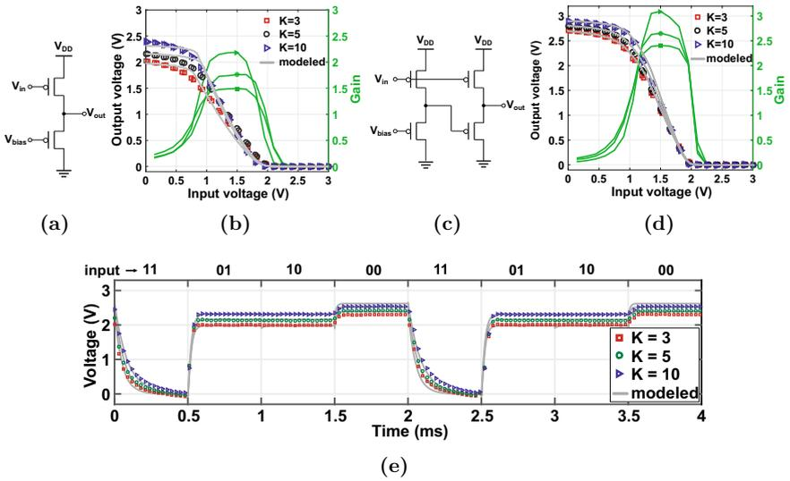
**Fig. 3.19** Schematics and measured vs. modeled voltage transfer characteristics of OTFT-based (a), (b) biased-load and (c), (d) pseudo-E inverters [76]. (e) Transient modeling and measurements of 2-input NAND gates based on biased-load inverter design. All OTFTs have a channel length of  $5\text{extmm}$
