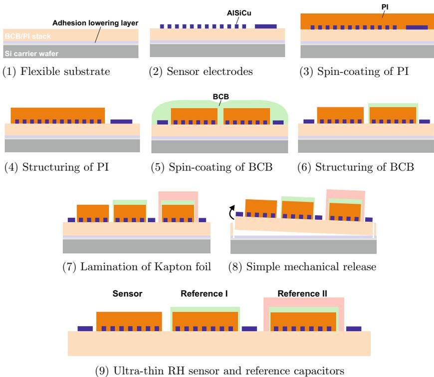
**Fig. 3.6** Fabrication process steps for the ultra-thin RH sensor, reference I and reference II. The sensing material is PI, which is isolated using BCB to fabricate reference I and an additional Kapton lamination to fabricate reference II. The foil is detached (cf. Fig. 3.7) from the carrier wafer for characterization
