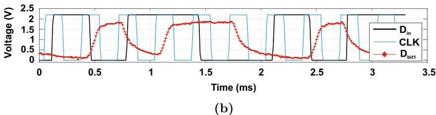
**Fig. 3.21** **a** Measurement and modeling of a 3-stage shift register operated using a supply voltage of 3V, bias voltage of -1V and clock frequency of 100 Hz. **b** Measurements of 1-stage shift register operated using supply voltage of 2.2 V, bias voltage of -1 V and clock frequency of 3 kHz
