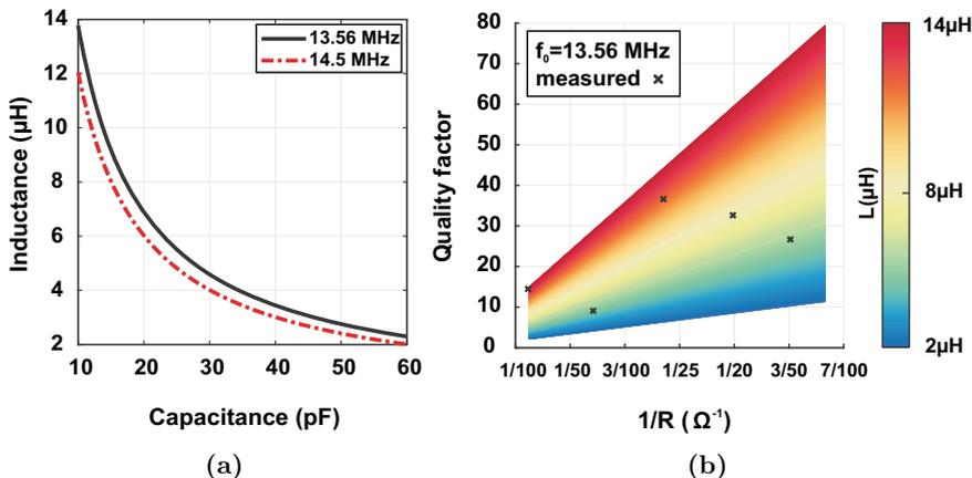
**Fig. 3.14** **a** Inductance value plotted against the required total capacitance for two NFC operating frequencies using equation 3.9. **b** Quality factor plane plotted against the loop equivalent conductance for different inductance values using equation 3.10 and some measured on-foil inductors are plotted
