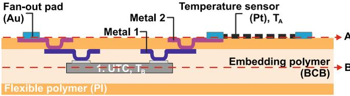
**Fig. 3.1** Cross-section of one variant of the CFP process in which embedded UTC and off-chip/on-foil temperature sensor are integrated into/on a flexible polymeric substrate [1]
