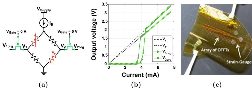
**Fig. 3.22** **a** Schematic of one strain gauge biased using current source and connect to a pair of OTFT analog switches. **b** Static measurements showing the performance of the OTFT analog switches in the off/on states. **c** OTFTs and printed strain gauges fabricated on the surface of the BCB/PI substrate [82]
