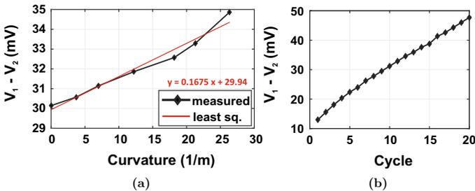
**Fig. 3.11** (a) Measurements show a monotonic increase of strain gauge output voltage with increasing the bending curvature [47–49]. (b) Bridge offset voltage increases after each bending cycle, until the memory effect is reset
