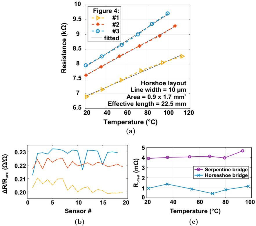
**Fig. 3.4** **a** Measured resistance of three RTDs with similar dimensions from three different setups. **b** Measured sensitivity of multiple RTDs from the three different setups shown in Fig. 3.3. **c** Bridge offset resistance  $R_{\text{offset}}$  plotted for Wheatstone bridge RTDs designed using serpentine and horseshoe layouts
