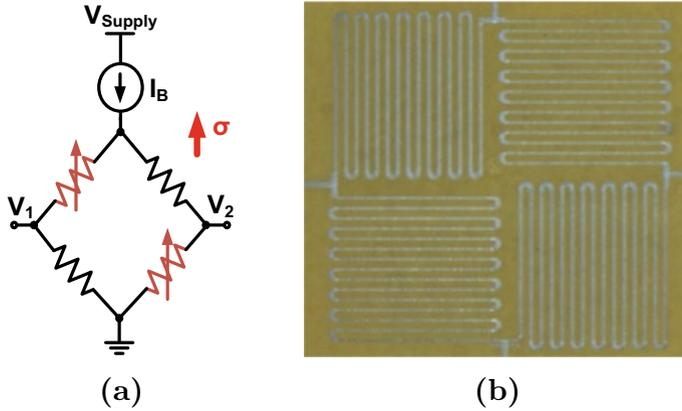
**Fig. 3.10** **a** Wheatstone bridge circuit, which has four resistors arranged in a diamond shape, biased using constant current source. **b** Photograph of serpentine-shaped strain gauge printed using silver ink on BCB/PI substrate. The linewidth is  $20\mu\text{m}$ , the total dimension of the bridge circuit is  $5 \times 5\text{mm}^2$  and nominal resistance of  $800\Omega$ . The direction of expected bending (i.e. mechanical stress  $\sigma$ ) of the robotic gripper is indicated
