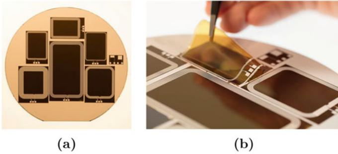
**Fig. 3.15** (a) Photograph of a test wafer for the fabricated on-foil spiral inductors using BCB/PI substrate [69]. (b) Photograph demonstrating the mechanical detachment of a spiral inductor from the carrier wafer
