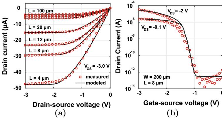
**Fig. 3.18** Measured and modeled static output and transfer characteristics of OTFTs
