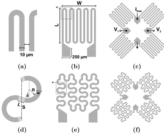
**Fig. 3.2** Temperature sensor design. **a–c** Serpentine and **d–f** horseshoe RTD layouts where minimum linewidth and spacing are  $10\ \mu\text{m}$ . Wheatstone bridge configuration using **(c)** serpentine and **(e)** horseshoe unit RTDs in which the resistance mismatch  $R_{\text{offset}}$ ,  $\Omega = (V_1 - V_2)/I_{\text{Bias}}$  is extracted
