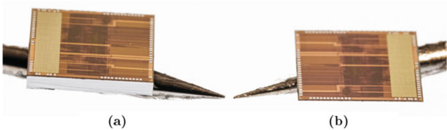
Fig. 4.17 Photographs of a 400- and b 30- \mu\text{m} thick low power microcontroller chips attached to probe needles for comparison
