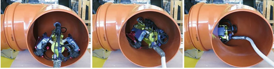
Fig. 2.6 Robot for pipeline inspection (Ciszewski et al., 2020)
