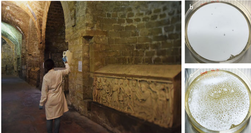
Fig. 2.3 Crypt environment. (a) Aerosol active sampling by portable sampler equipped with sterile disposable gelatine filter; (b) nutrient medium inoculated by Gelatine filter (completely water-soluble); (c) dissolving of gelatine filter during the contact with Nutrient Agar (the filter completely disappears in a few minutes)
