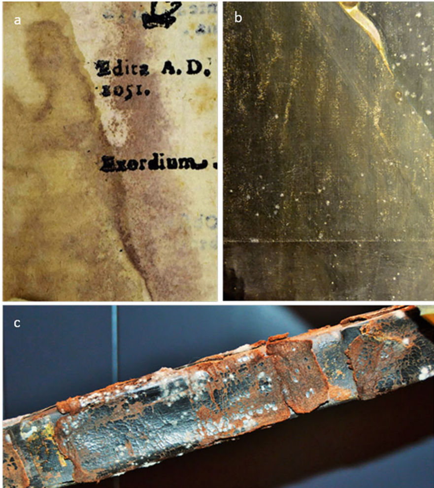
Fig. 1.3 Microbial colonization on organic materials: (a) paper document affected of pigmented spots originated by microorganisms, (b) an oil painting on canvas with fungal colonization on verso and (c) a lather sword holder completely damaged by white fungal colonization
