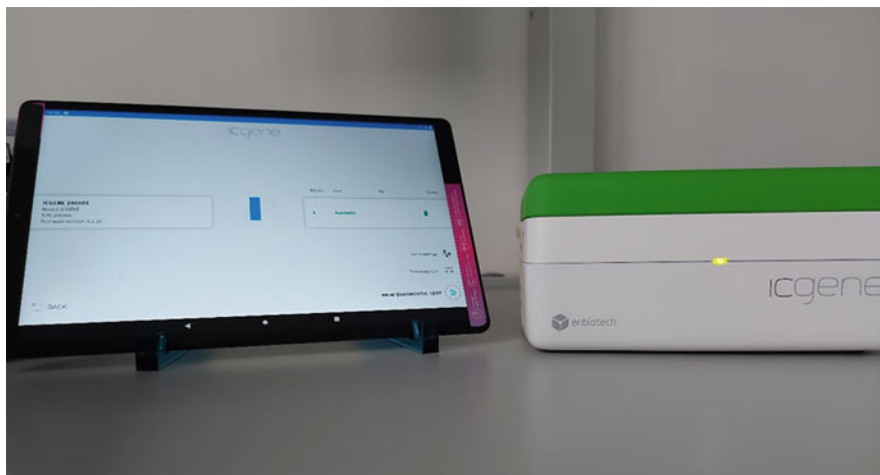
Fig. 5.6 LAMP technology. ICGENE portable mini instrument. The amplification profiles specific for bacteria or fungi cells can be directly followed on wireless connected tablet. ICGENE is a high sensitive, specific and easy-to-use in vitro diagnostic device able to perform the amplification of DNA target sequences in few minutes. The LAMP technology includes a portable fluorescent reader by measuring of light emission of analysed sample, which provides step-by-step assistance in performance of analysis by the use of an intuitive front-end (tablet and app)
