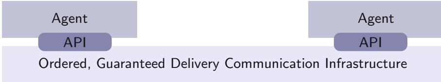
Fig. 2. MAS where agents communicate via a reliable infrastructure that guarantees message delivery and in FIFO order.
