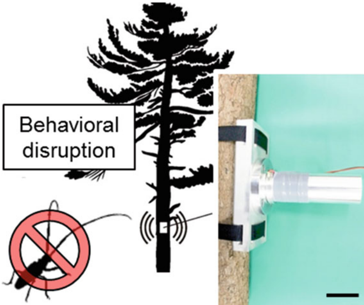
Fig. 20.8 A schematic of the vibrational pest control procedure. A vibration exciter made with giant magnetostrictive materials is attached to a tree, and it generates vibrations to disrupt behaviors of insects. Scale bar = 50 mm. Adapted from a photo of Takanashi et al. (2019)
