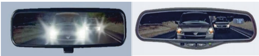
Fig. 11.2 Conventional mirror (left) causing glare of reflecting lights and mirror ultrathin coating with nanocomposite (right) making it glare-free. (Source: Mathew et al. (2019))
