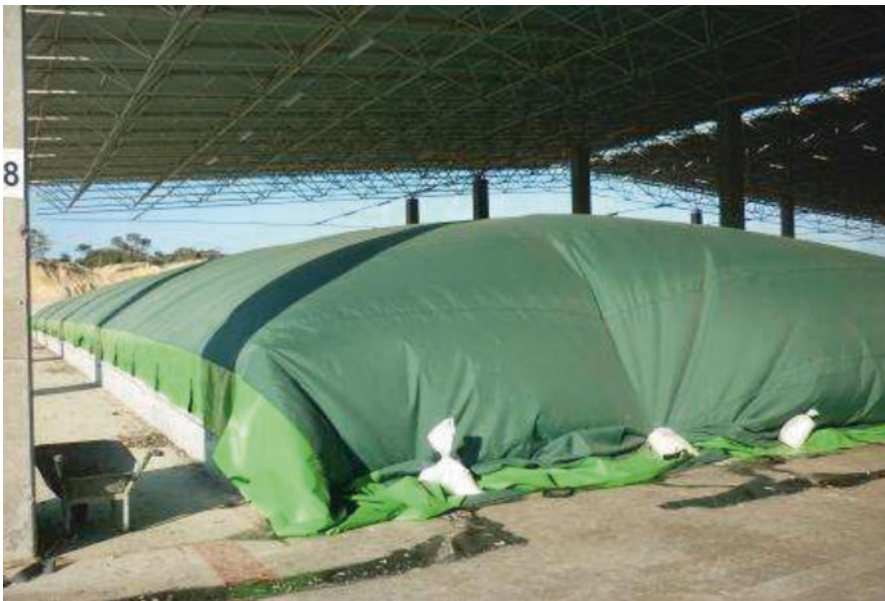
Fig. 7.31 Waste heaps covered with a geotextile membrane
