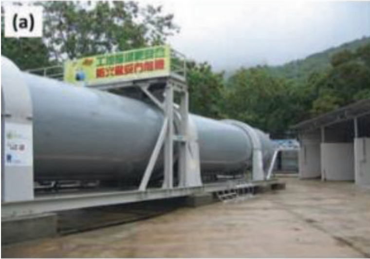
Fig. 6.20 In-vessel composting in rotary drum composter [4]
