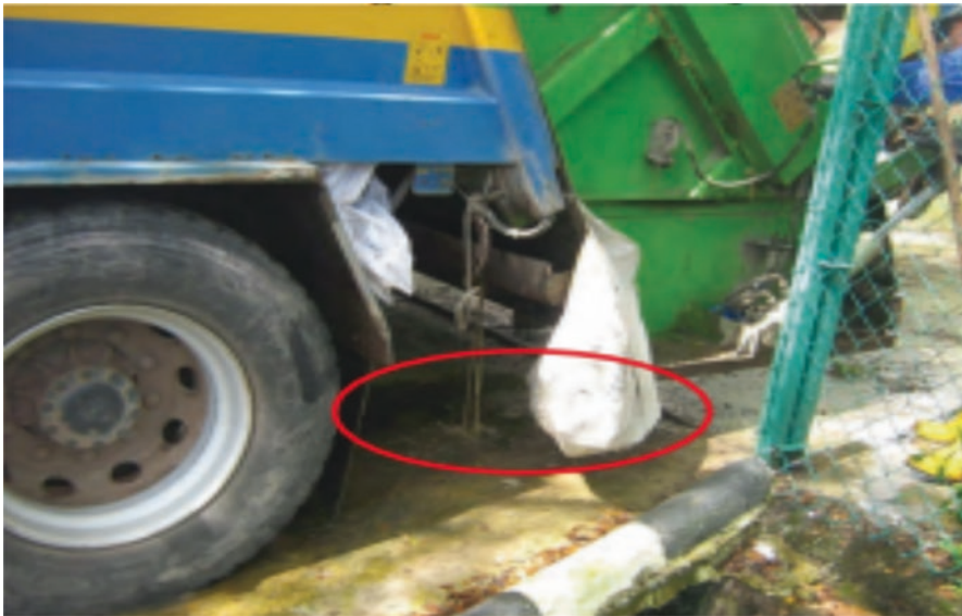
Fig. 7.40 Leachate spillage from a compactor truck
