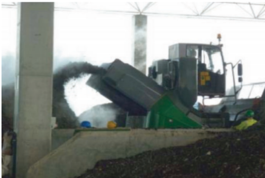
Fig. 7.32 Turning process using machine
