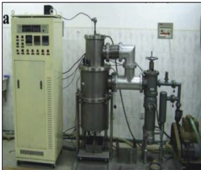
Fig. 3.9 Illustration of the vacuum recovery system for distillation [28]
