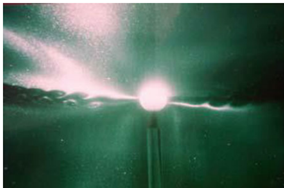
Fig. 10 Direct photograph of swirling equatorial disc outflow (DO) created by a rotating rigid sphere in otherwise stationary silicon oil with aluminum powder illuminated by laser sheet [132]
