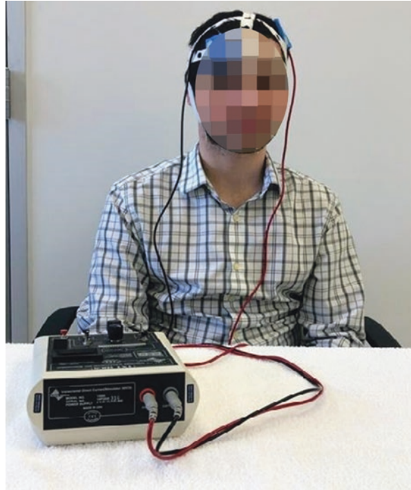
Fig. 14.1 Common setup for transcranial direct current stimulation
