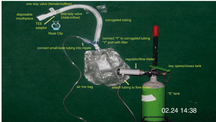
Fig. 1 CO 2 delivery system without capnometry in place – Original delivery system developed by Brenda Rinsky, RDMS, RVT, NVS
