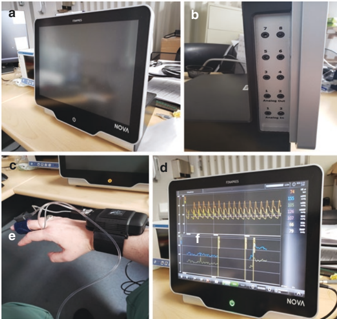
Fig. 3 Non-Invasive Continuous Full Waveform ABP Monitoring Device. ABP arterial blood pressure. (Panel a ) Photo of the Finapres NOVA non-invasive ABP monitor, (Panel b ) Photo of analogue output ports on Finapres NOVA system, allowing full integration with other bedside monitoring and data acquisition platforms, (Panel c ) Examples of wrist mounted and fingertip based ABP monitoring system, (Panel d ) example of continuous full waveform non-invasive ABP monitoring
