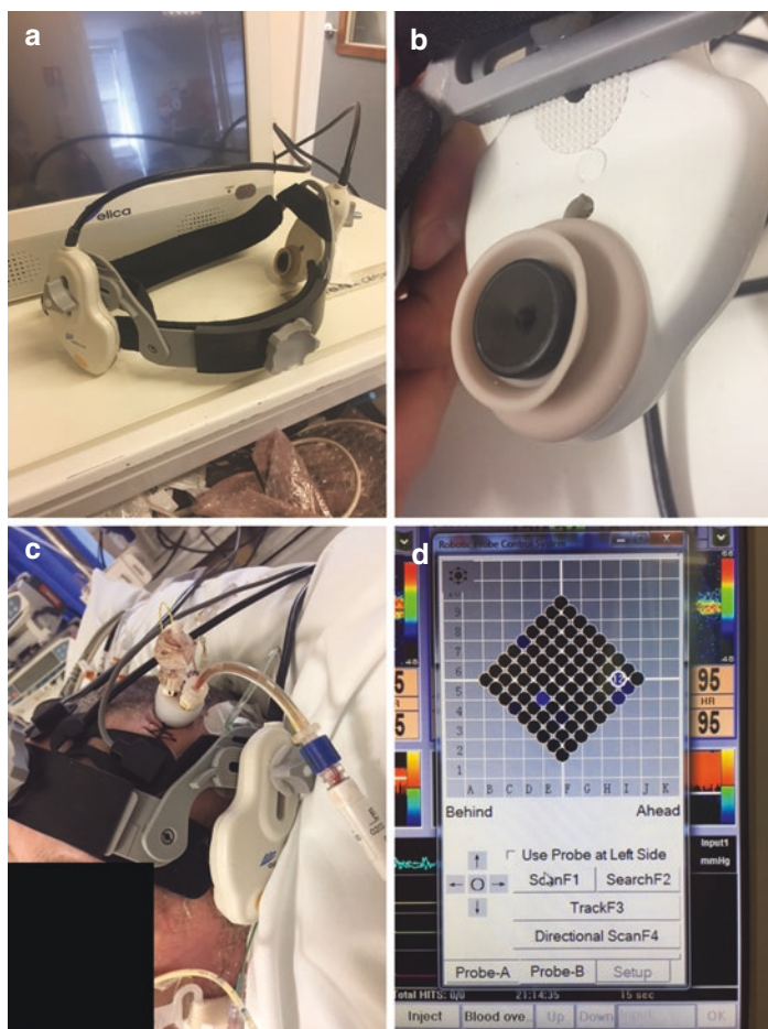
Fig. 2 Robotic TCD Device Example. TCD transcranial Doppler. (Panel a ) Displays robotic TCD headframe with two robotic drives mounted to a ratcheting headband system. (Panel b ) displays close up image of TCD probe encased in robotic drive. (Panel c ) example of set up for multi-modal monitoring with left frontal triple bolt, (Panel d ) Delica EMS 9D TCD program display, showing automatic flow velocity sampling algorithm, producing a square grid of sampled insonation positions. The system insonates at multiple sites, finding the area with superior signal quality). (*Figure is a color adaptation from Zeiler et al. (with permission from corresponding author) [47])
