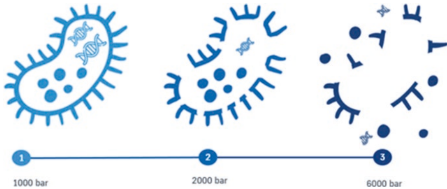
Fig. 15.2 Inactivation of microorganisms in relation to applied pressure (Anonymous 2020)
