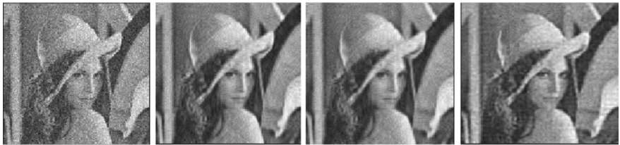
Fig. 11. Lena: From left to right noisy image, DCT, TMs, and KMS denoised images.
