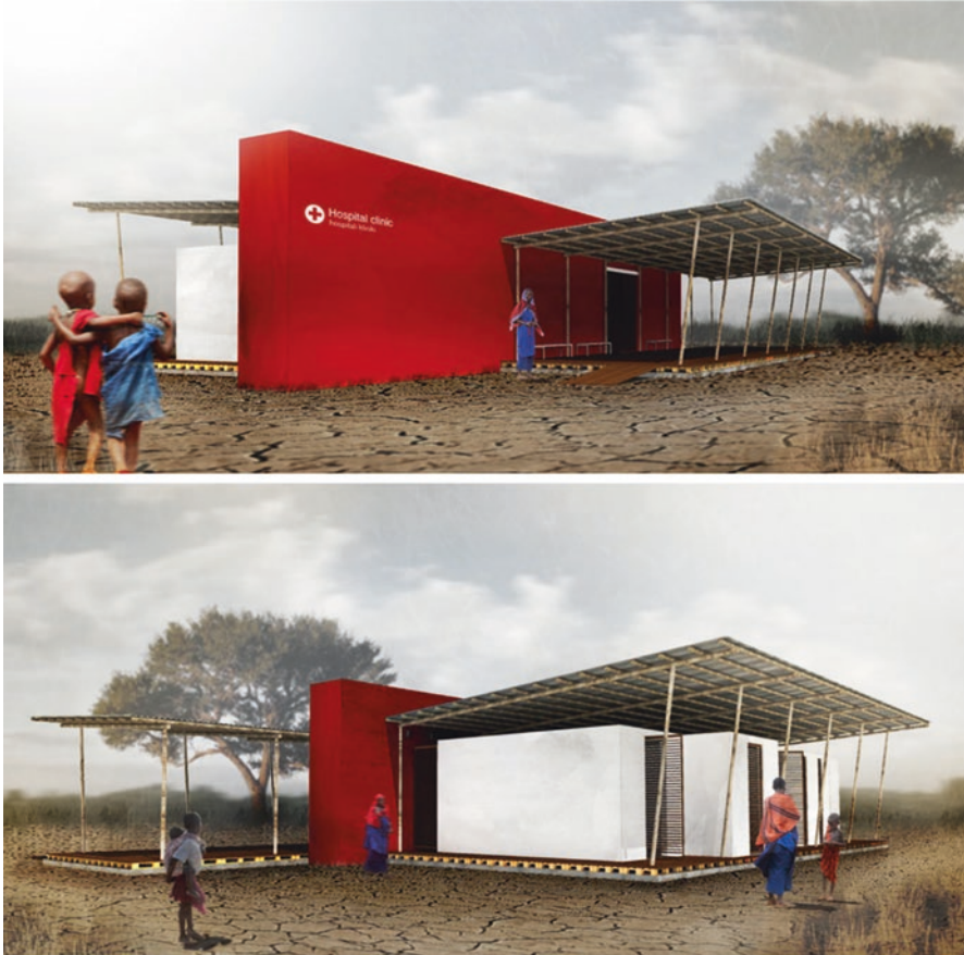
Fig. 14.2 views of the dispensary of Chakama. Note the central red volume, which houses the power plants
