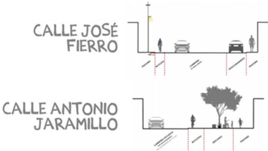
Fig. 23.5 Street section of the team proposal at Jose Fierro and Antonio Jaramilla Streets (image by team)
