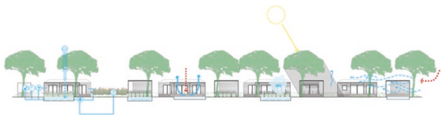
Fig. 15.4 Section highlighting environmental compensation and sustainability: water collection and phytodepuration, natural ventilation, air cooling through water, natural shading, O 2 production (Credit: AUDe Lab, University of Pavia)
