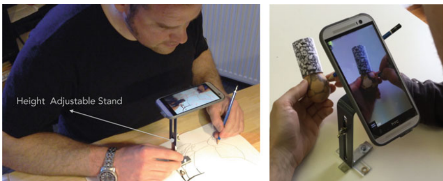
Fig. 18.8 Mobile device renders a virtual template image together with a live video stream of the drawing surface. Left: paper. Right: Easter egg
