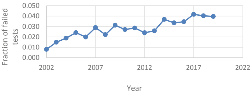
Fig. 1. Fraction of DHSV failures on number of tests
