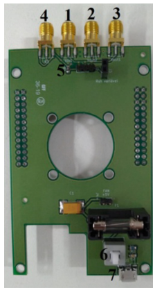
Fig. 3. Measurement circuit. 1: SMA connector for input signal; 2: SMA connector for channel 1 output signal; 3: SMA connector for channel 2 output signal; 4: SMA connector to device under test connection; 5: Shunt resistor; 6: Button on/off; 7: Micro USB power.
