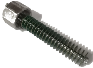
Fig. 1. Prototype of the capacitive sensor developed in [5].
