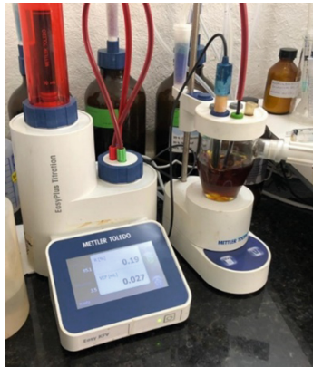
Fig. 5. Karl Fischer titration of one sample of oil.
