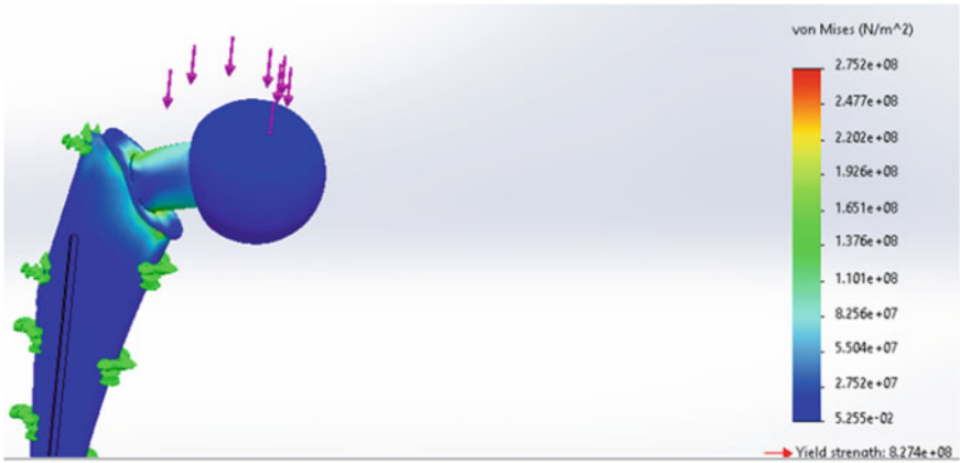
Fig. 5. Stress Von Misses yield for an applied force of 2044 N.
