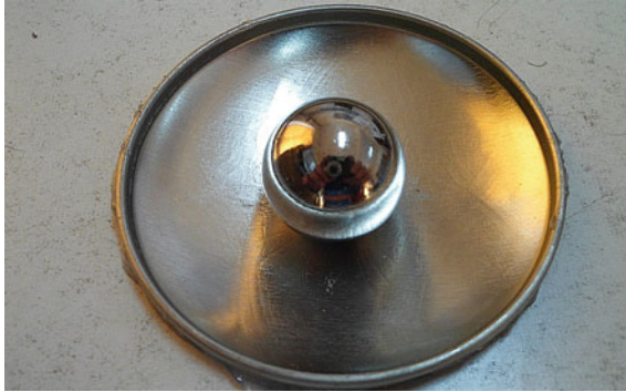
Fig. 2. Experimental model of rolling pendulum system (RPS)
