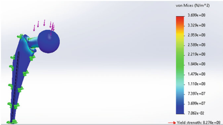
Fig. 7. Stress Von Mises yield when applying a force of 2747 N.
