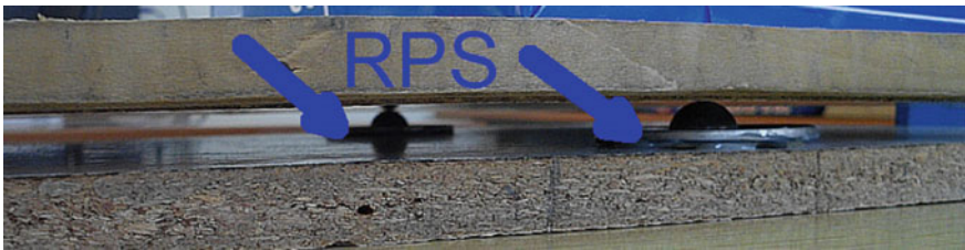
Fig. 3. The experimental stand with rolling pendulum system mounted
