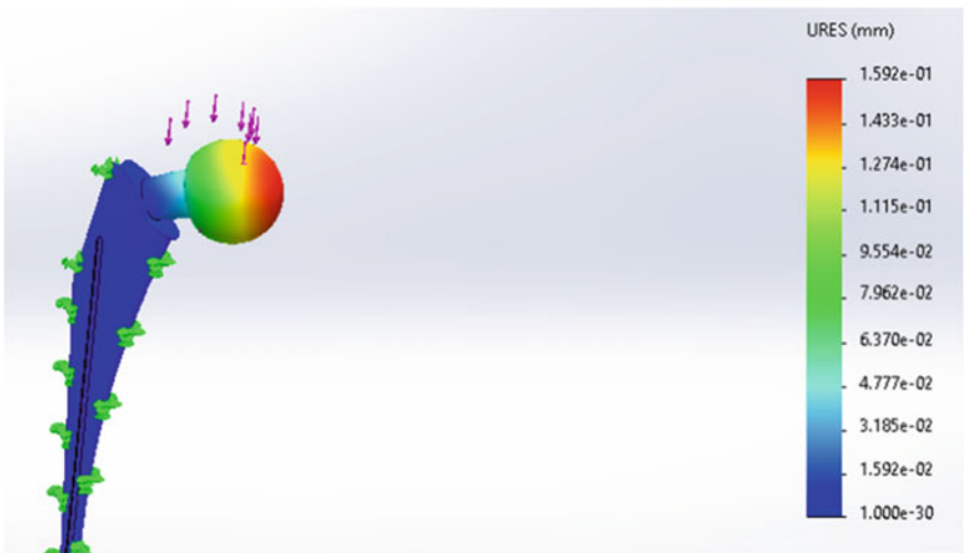
Fig. 6. Visualization of displacements (URES) when applying a force of 2044 N.
