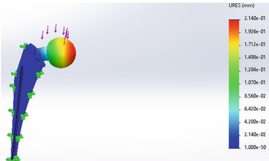
Fig. 8. Visualization of displacements (URES) when applying a force of 2747 N.
