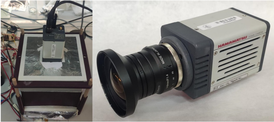
Fig. 4. InGaAs camera, Hamamatsu brand and C12741-11 model, for EL imaging.
