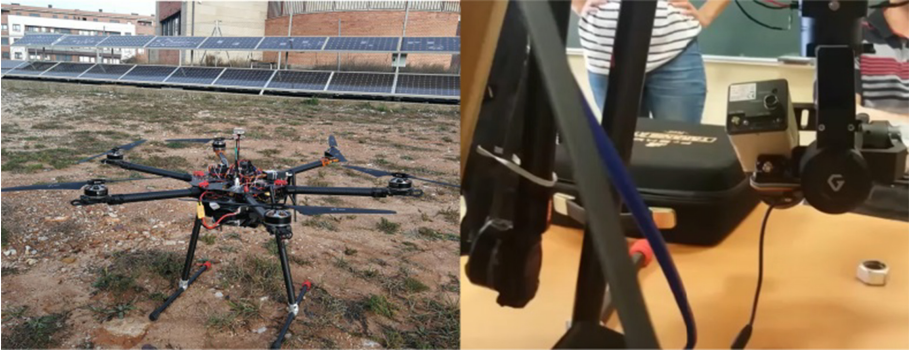
Fig. 3. Drone and InGaAs camera installed on gimbal.
