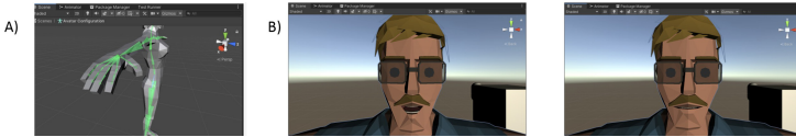
Fig. 4. Use of animation. A) Skeleton for avatar animation. B) Facial animation using blendshapes. Pronouncing letter O (left) and letter T (right)
