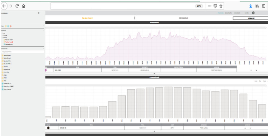
Fig. 11. View of the information that is recorded in the SEEDS system on the electricity consumption (KWh) of CIDETEC on a particular day, in this case 01/22/2019.
