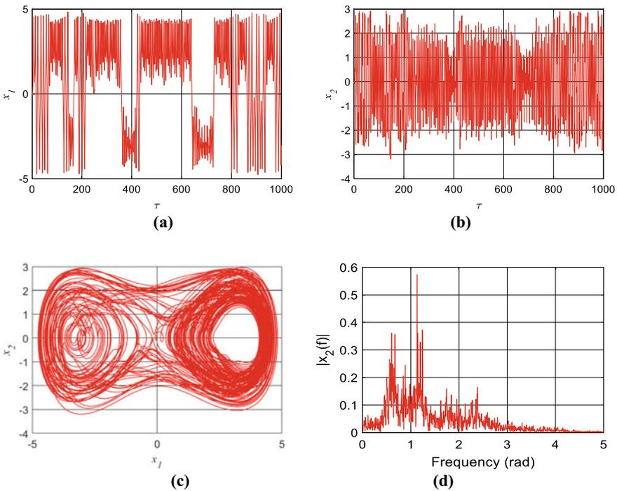
**Fig. 3** **a** Time history of the states  $x_1$ . **b** Time history of the states  $x_2$ . **c** Phase diagram to  $x_1$  versus  $x_2$ . **d** Power spectral density (FFT) to  $x_2$
