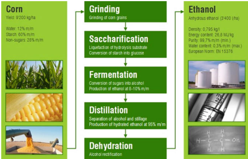
Fig. 4 Process of Bioethanol production (Janke et al. 2015)
