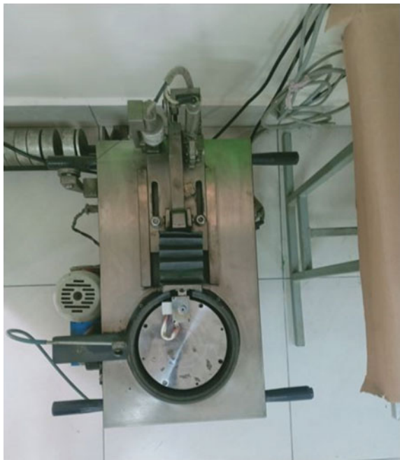
Fig. 3 Top view of the pin on disc tribometer with showing counter surface and pin holder
