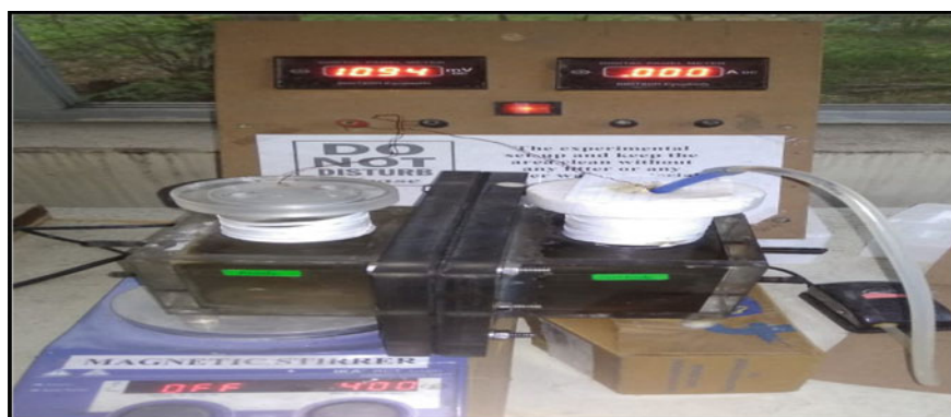
Fig. 2 Experimental setup of microbial fuel cell
