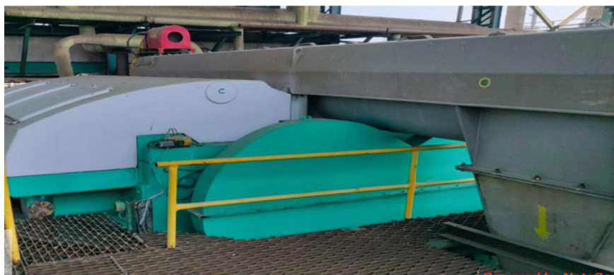
Fig. 3 New generation twin roll press for pulp washing
