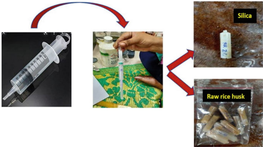
Fig. 2 Method for the preparation of pin sample
