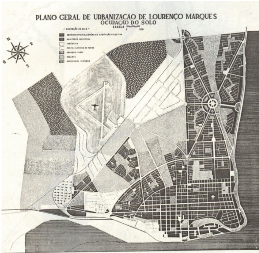
Fig. 4 Maputo general urban expansion ‘Aguiar Plan’ of 1952, showing the primary planned expansion to the northeast, avoiding most existing unplanned ‘reserves’ to the northwest. Source author’s personal archive
