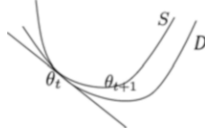
Fig. 12.10 Reprinted with permission from [95]. The surrogate S majorizes (upper bounds) D , and they touch each other at \theta_t with the same tangent
