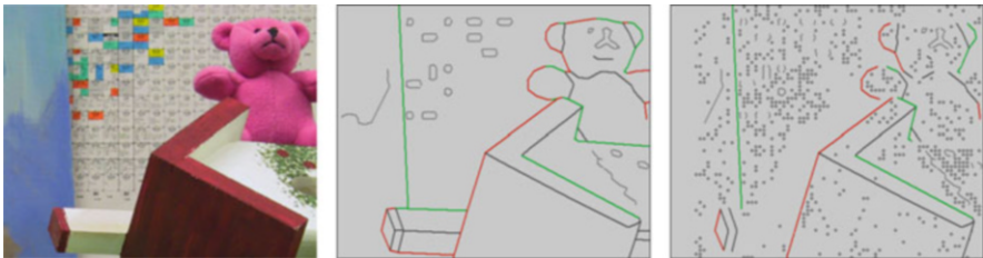
Fig. 8.11 Reprinted with permission from [4]. Left image of a stereo sequence, the graph labeling, and the control points (point and boundary primitives) of the thin plate spline
