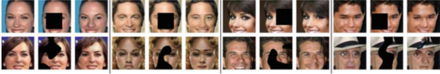
Fig. 11.8 Reprinted with permission from [69]. Inpainting examples on CelebA dataset. In each block from left to right: the original image, masked input, inpainted image by the multi-grid method
