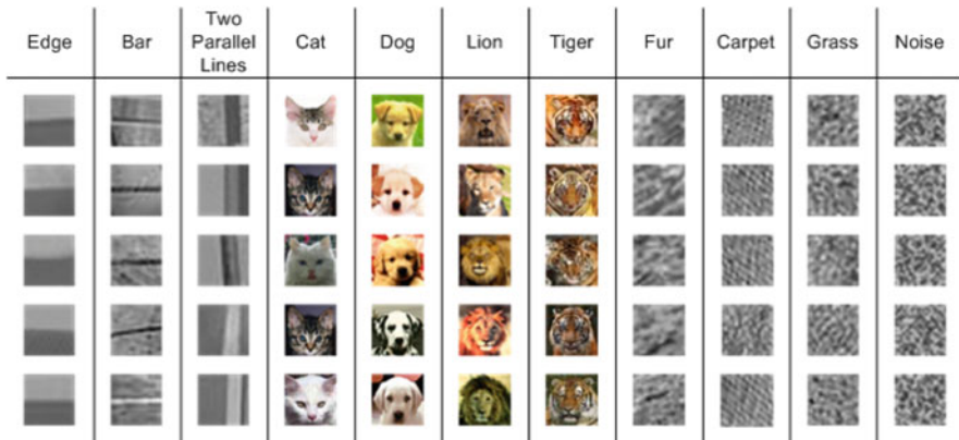
Fig. 1.8 Simple geometric patterns like edges and bars have low entropy, while stochastic textures like fur and carpet have high entropy
