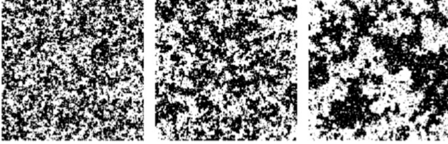
Fig. 3.5 Example sampling of Ising Model with different mean and variance. From left to right, \beta is 0.35, 0.40, and 0.43, respectively
