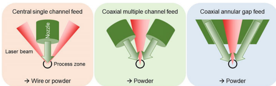
Fig. 10 Nozzle design for coaxial laser material deposition and typical applications: central single channel feed for use of wire or powder (left), coaxial multiple channel feed (middle) and coaxial annular gap feed (right), both used for powder only
