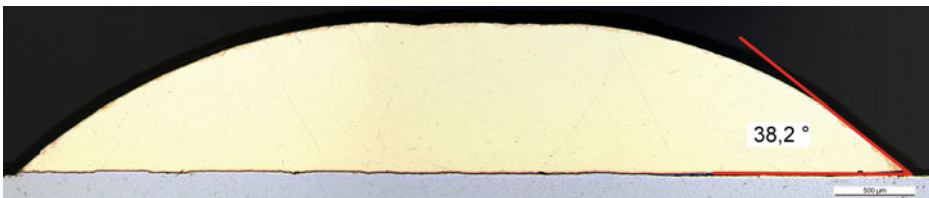
Fig. 6 Microstructure of wetting of pure copper on molybdenum substrate
