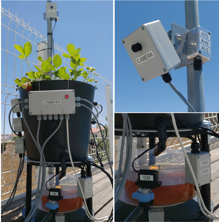
Fig. 8. Prototype appearance and some hardware details (right figure).
