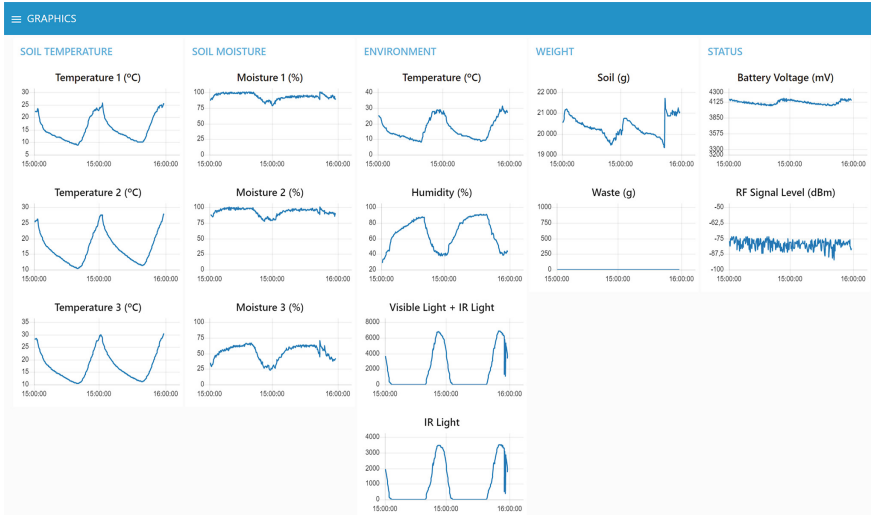
Fig. 11. NodeRed dashboard with graphs of the last 24 h data.
