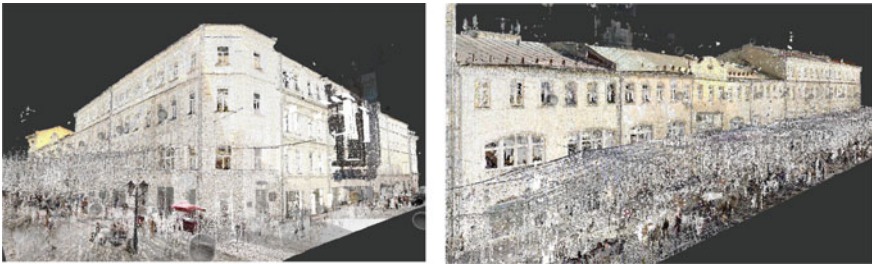
Fig. 6 An example of a digital model of CHO in the form of a point cloud (Source: materials of the restoration project of JSC “Guta-Development”)
