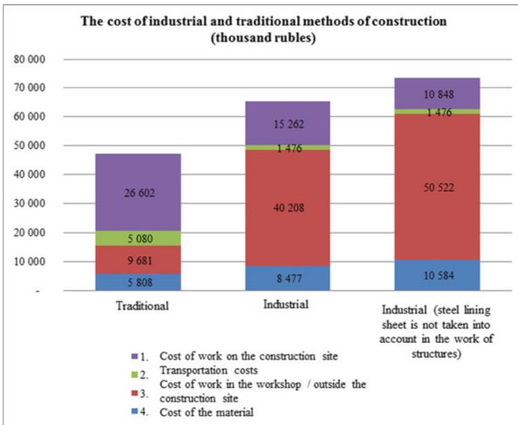
Fig. 2 Comparative cost when performing reinforcement and shuttering works by industrial and traditional methods
