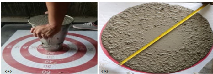
Fig. 1 a Abrams cone filled; b Scattering measurements
