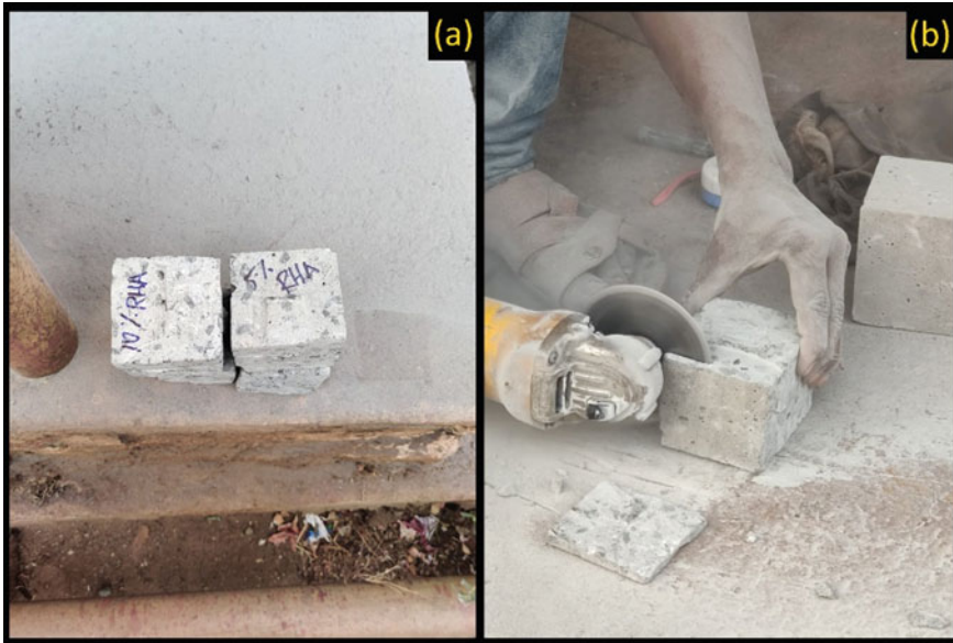
Fig. 1 a Exposed core b Cutting of specimen
