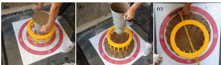
Fig. 3 a Positioning and filling the cone; b Suspension; c Measurement of diameters
