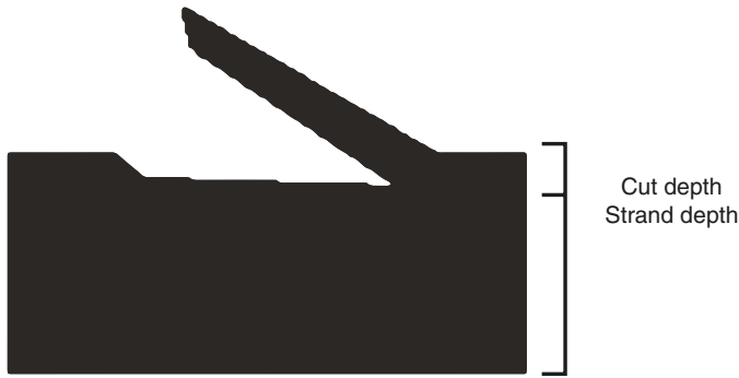
Fig. 9.12 Barb of bidirectional thread
