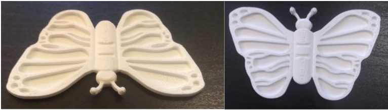
Fig. 2. A butterfly printed with a ZYYX+, layer 0.15 mm, material PLA
