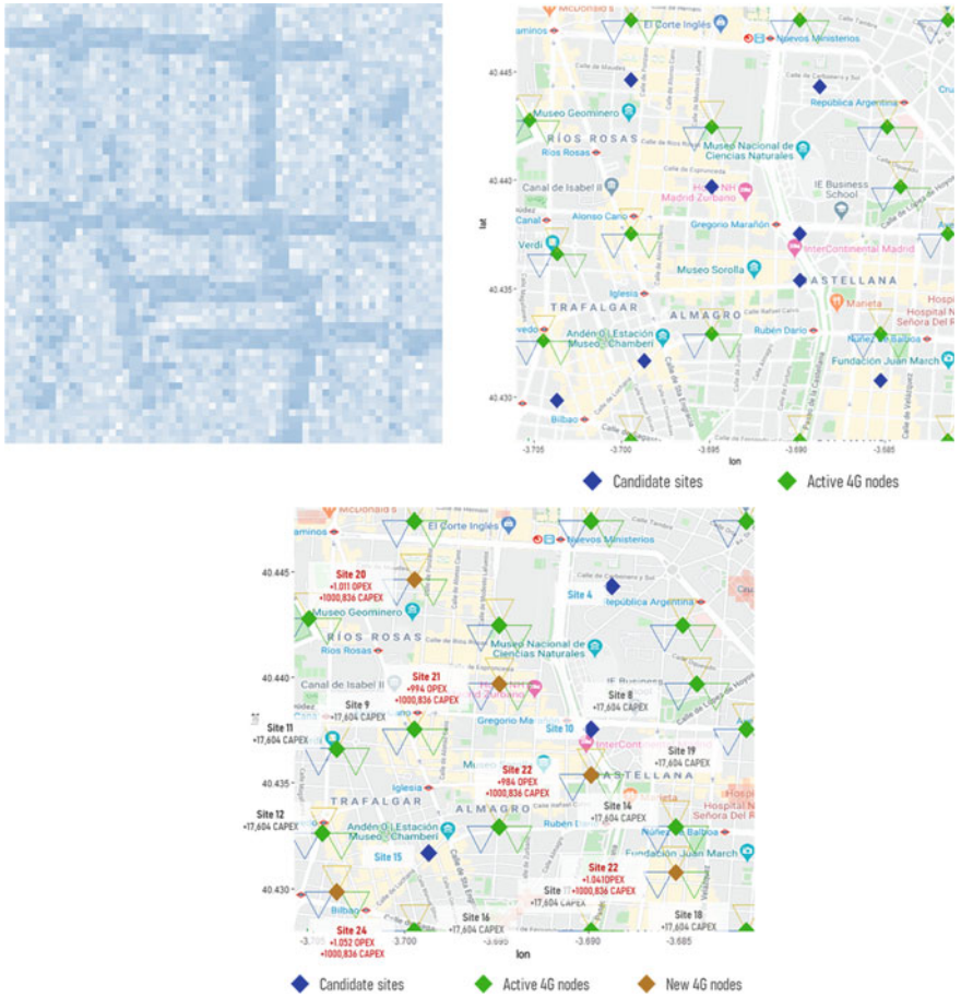
Fig. 15.2 Traffic demand (top left) and current network plan (top right) maps. Optimal network plan map (bottom)
