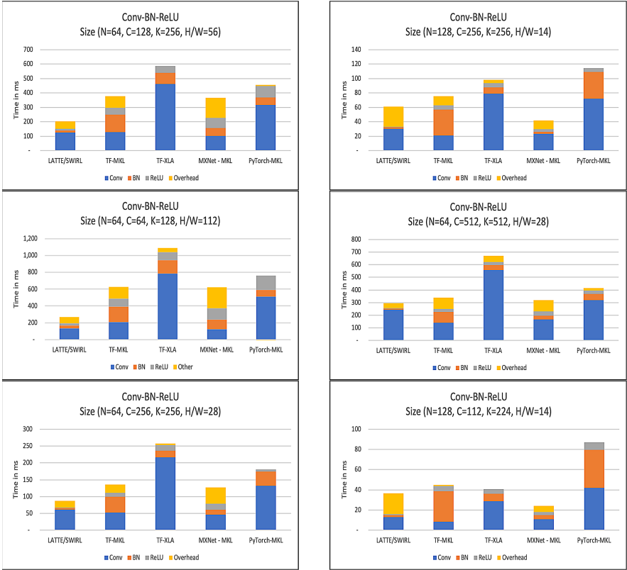
Fig. 10. Performance results in time (ms) for the Convolution-Batch Normalization-ReLU layer training step. Displays the time spent on each operator.
