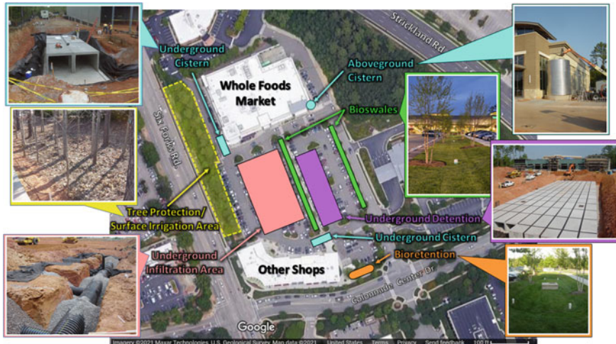
Fig. 4 Layout of green infrastructure practices used to mitigate the quantity and quality of stormwater for the Market at Colonnade development (Aerial image procured from Google Maps; photos taken by Soil & Environmental Consultants, PA and Regency Centers)
