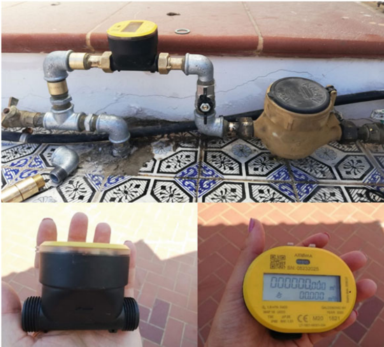
Fig. 7 High-resolution measurement and traditional water metering at the pilot site. Source Authors
