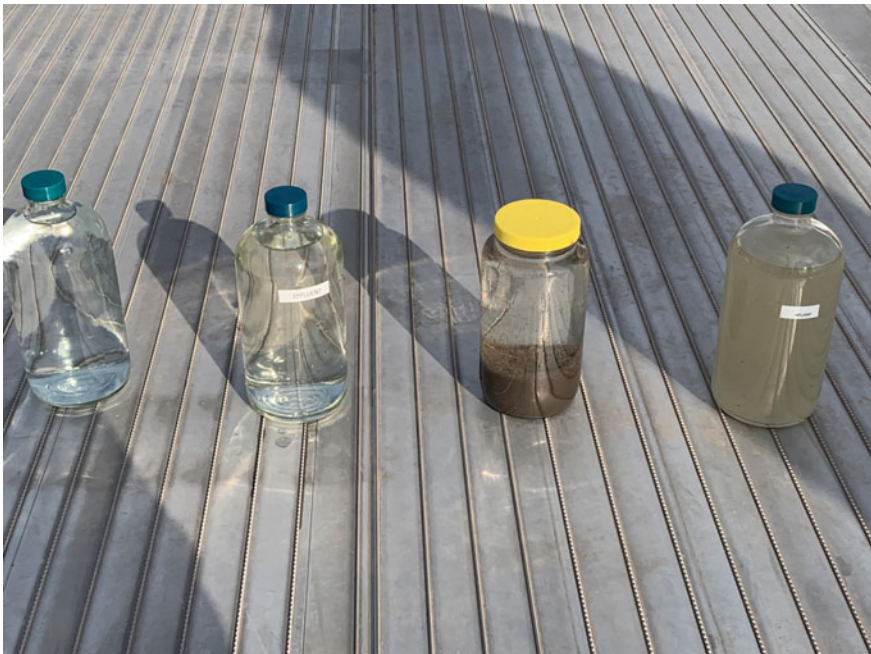
Fig. 3 An example of the visual educational elements of the tour. From left to right; Norman tap water, plan effluent after treatment and disinfection, wastewater after primary clarifier, wastewater after preliminary treatment. Source Author
