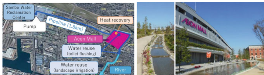
Fig. 3 Schematic diagram of the supply of reclaimed water to Aeon Mall Sakai Teppocho [6, 7]
