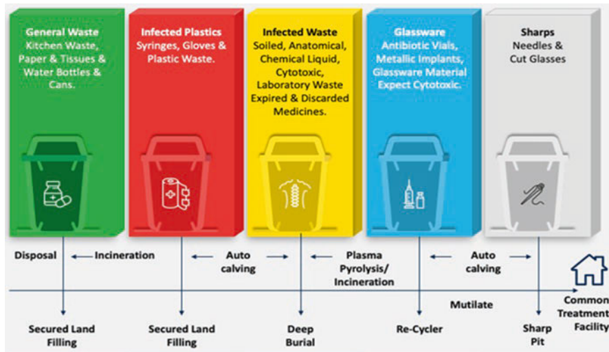
Fig. 2 Segregation of hospital biomedical wastes. (Source: Patan & Mathur, 2015)
