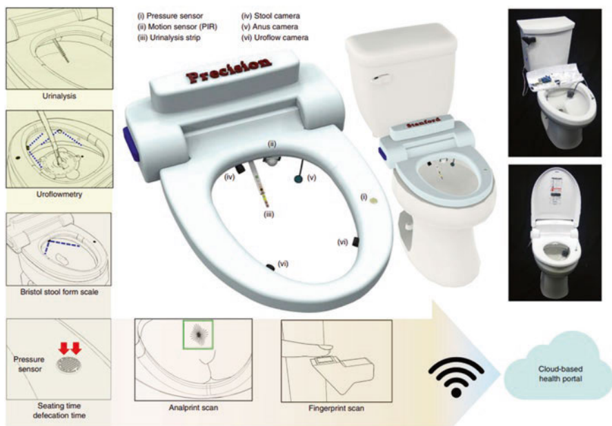
Fig. 4 Mountable smart toilet. (Park et al., 2020)
